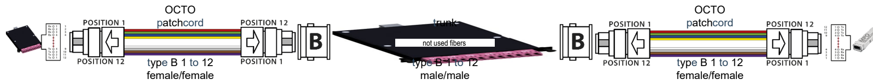
patchcord and trunk IEC fiber color code / MTP® adapter B „aligned keys“ „1 to 12“
